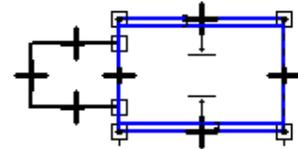
17. Select the bottom horizontal, blue line of the plan view. Right mouse click to activate the Tick button on the ribbon bar and click a point above the line just selected. Click the right mouse button to reset the command.
