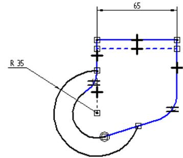
14. On the ribbon bar, click the Diameter
