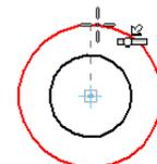
16. Type "25 mm" in the Length box (this should already be highlighted, so just type in the value directly) and press the TAB key. Type "90" in the Angle box and press ENTER.
