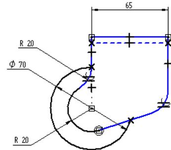
18. Move the mouse cursor slightly up and to the left to position the dimension and click to place.
