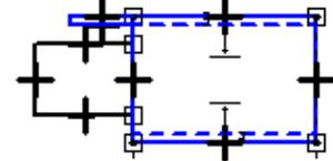
21. Click the Tangent relationship button. Click the 3mm vertical line just placed (to select the correct line, hover the cursor over the line and wait for Quickpick to display and then right mouse click to see each of the lines highlight) and then click the 20mm inner arc in the front view. This should adjust this profile to match the front view.
