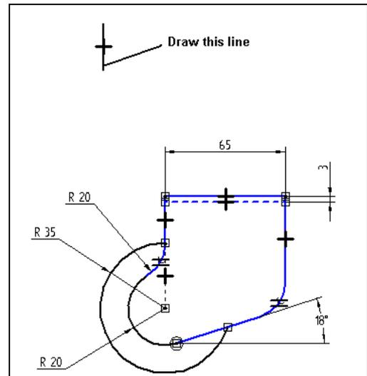
5. Click the Line button and place the first point at the bottom end of the vertical line just placed.
