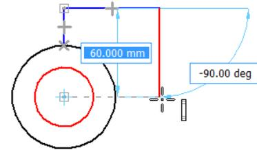
19. Move the mouse cursor to the bottom of the inner circle. Click when the point on and tangent indicators are displayed. Click the right mouse button to exit the line command.
