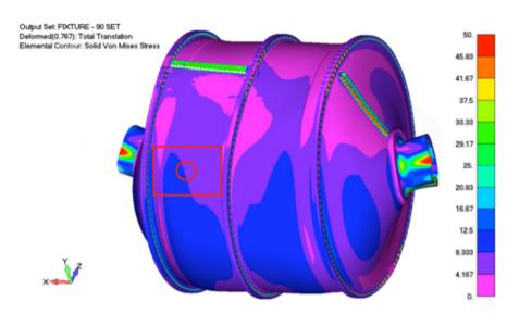
A "ball port" (=hole) is sometimes required in the cylindrical barrel of the mill. This local design detail can be considered without re-running the entire mill model, by using sub-modelling.
