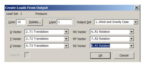
Then Femap asks for the nodes to which the enforced displacement loads are applied, which are obviously all the nodes at the external boundary(ies) where the sub-model is connected to the rest of the global model.
