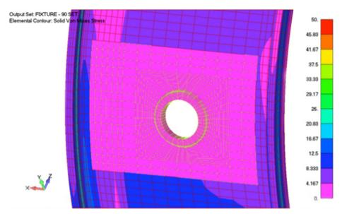
Above: Continuous mesh in the cylindrical barrel, replaced by local mesh including hole and local reinforcement (hence zero stress in the local mesh).
