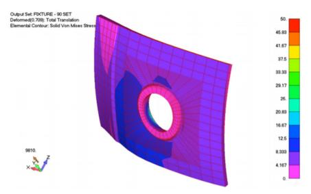
Results from local model of ball port (corresponding to load/result set shown in previous image).
