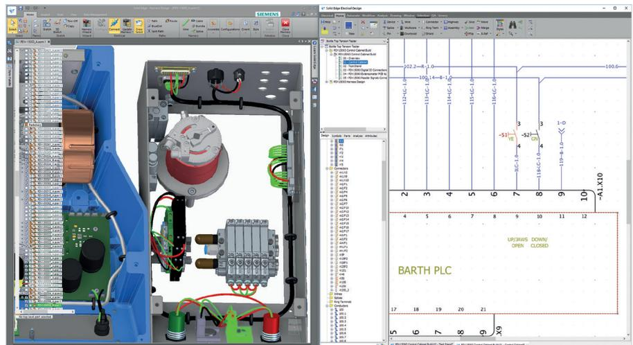
Solid Edge Electrical Routing directly interfaces between Solid Edge Wiring and Harness Design using a feature called connected mode, which allows the user to bridge environments and update harness information.
