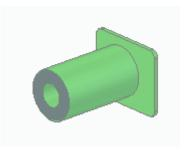
The final setting available is the "Remove voids" option, just below half way down the options. When we turn this on, any internal geometry is also removed.
