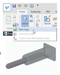
If we change the settings by turning on the "Adjust non-manifold conditions and merge" option, the result is that it adds a little overlap of material, thus joining the bodies. If we use the clipping planes though, you will see that some of the internal geometry is still visible.
